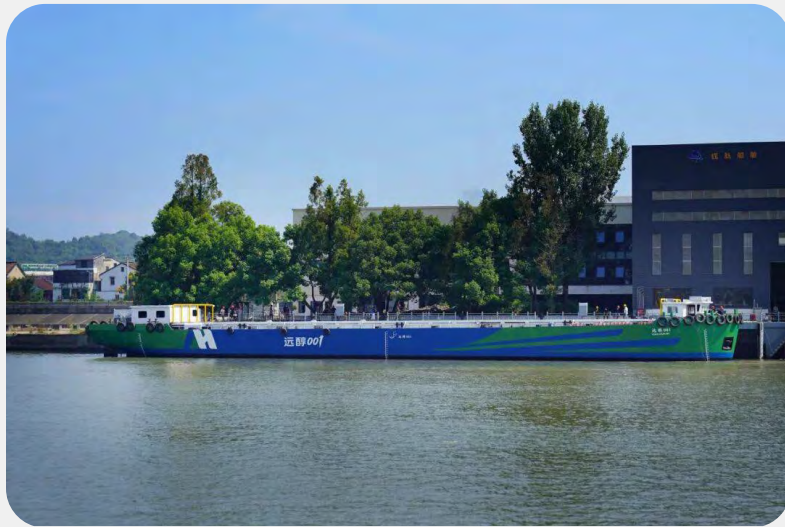
World's first methanol-hydrogen electric general cargo-passenger ship
